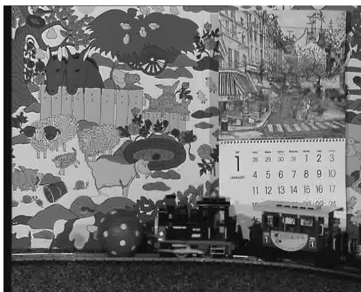
Figure 6-12 The "mobile" sequence MPEG2 compressed to 2Mbps: it is easy to spot the blocking artefacts even on a still frame.
